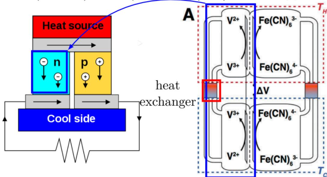
Figure 4: Continuous electrochemical heat engine. Convert **heat** into electric energy.
