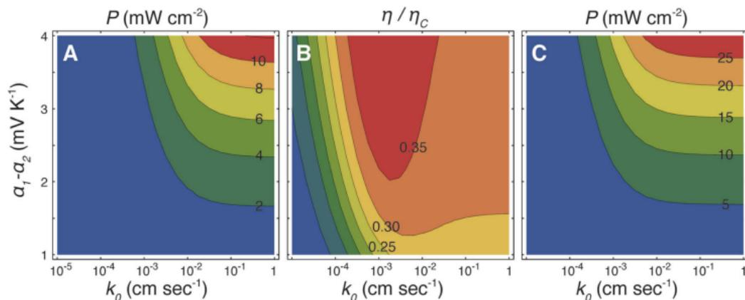
**Figure 10:** Simulations of **liquid-based** continuous electrochemical heat engines. Maximum power density (A) and efficiency at the maximum power point (B) for a heat engine operating between 50 °C and 10 °C as a function of redox-active fluid properties  $\alpha$  and  $k_0$ , with concentrations of active species corresponding to the experimental system. (C) Concentrations of activate species increased to 15M.
