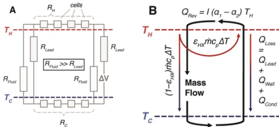
Figure 6: Electrical and thermal irreversibilities in the continuous electrochemical heat engine.
