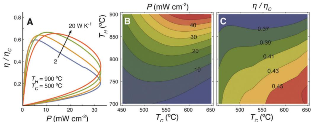
**Figure 9:** Simulations of **gas-based** continuous electrochemical heat engines. (A) Efficiency and power parametrized by the current-voltage curves. The four curves correspond to a counterflow heat exchanger rated for 2, 5, 10, and 20 W K<sup>-1</sup>. (B)-(C) Maximum power density and efficiency as a function of  $T_H$  and  $T_C$ .
