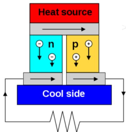
**Figure 1:** A thermoelectric circuit composed of materials of different Seebeck coefficients (p-doped and n-doped semiconductors), configured as a thermoelectric generator.
