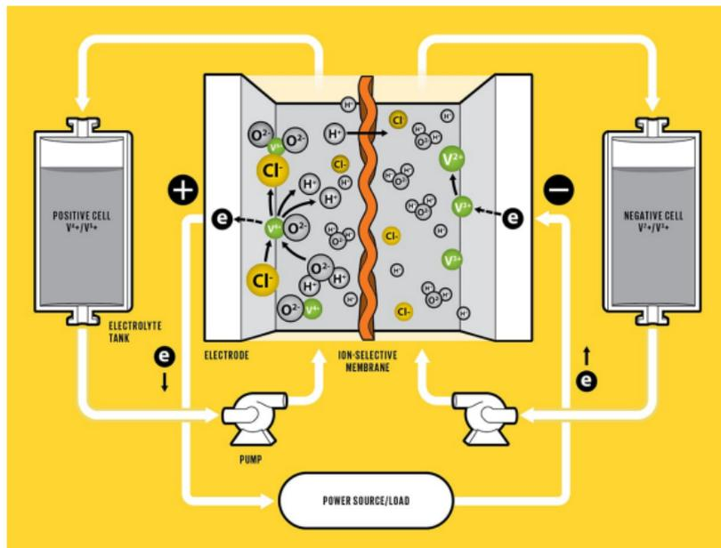
Figure 3: The Vanadium Redox-Flow Battery.
