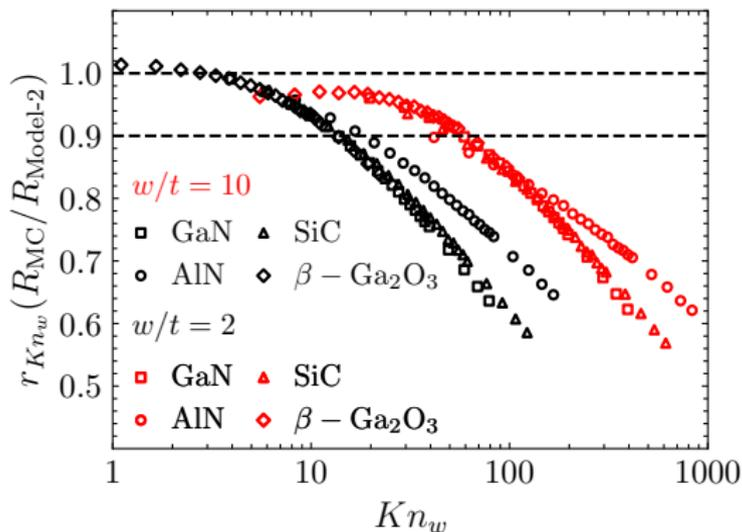
Figure 8: Thermal resistance ratio as a function of  $Kn_w$ .
