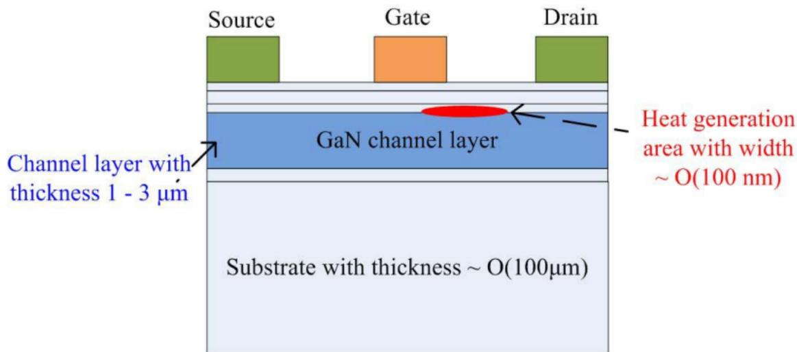
Figure 1: Typical structure of GaN HEMTs.
