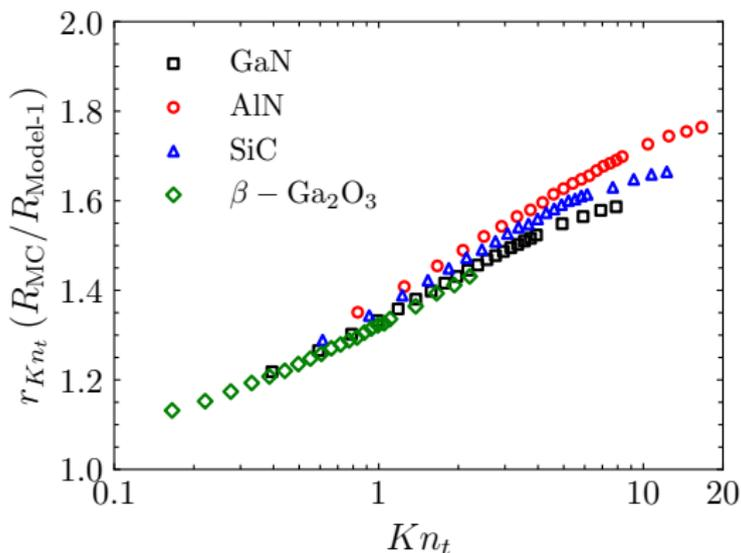
Figure 6: Thermal resistance ratio as a function of  $Kn_t$  of different materials.
