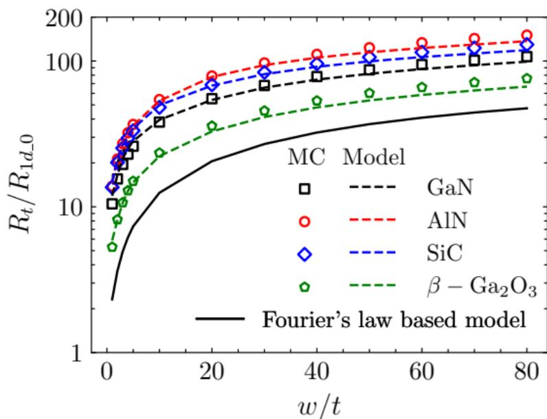
Figure 10: Dimensionless total thermal resistance of Different semiconductor materials as a function of  $w/t$  with  $w_g/w = 0.01$  and  $t = 2.7 \mu\text{m}$ .
