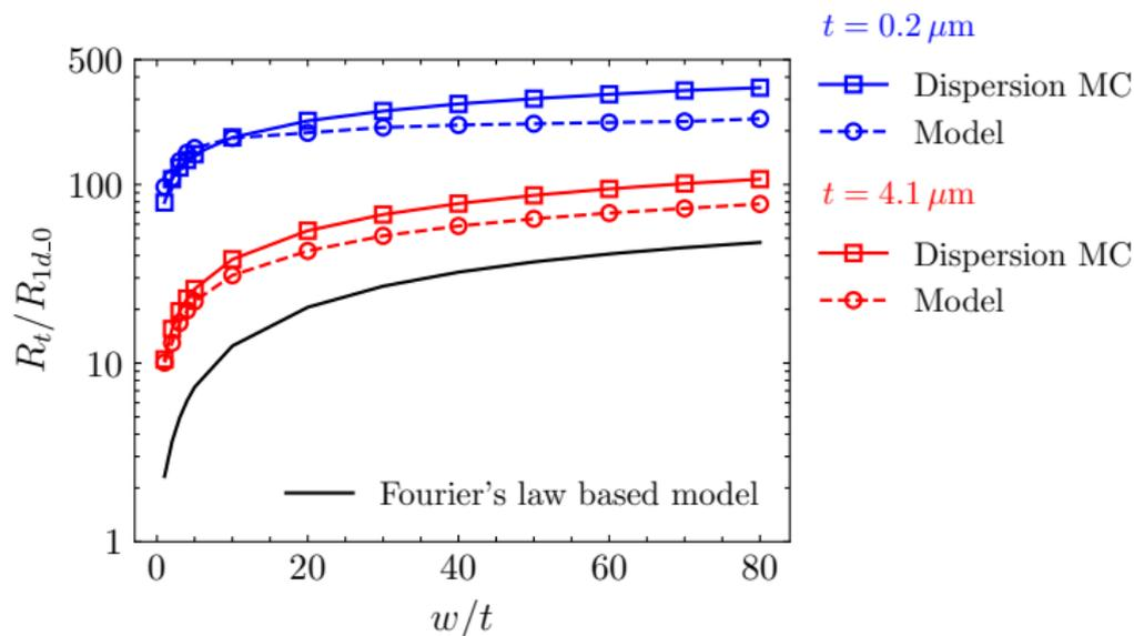
Figure 4: Dimensionless total thermal resistance of GaN as a function of  $w/t$  with  $w_g/w = 0.01$  under different thickness.
