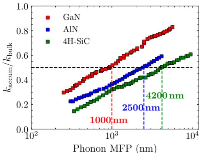
**Figure 3:** Normalized thermal conductivity accumulation functions of GaN, AlN, and 4H-SiC at temperatures near 300 K as a function of phonon MFP.<sup>3</sup>
