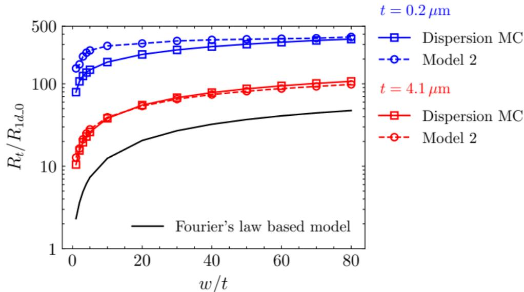
Figure 7: Dimensionless total thermal resistance of GaN as a function of  $w/t$  with  $w_g/w = 0.01$  under different thickness.
