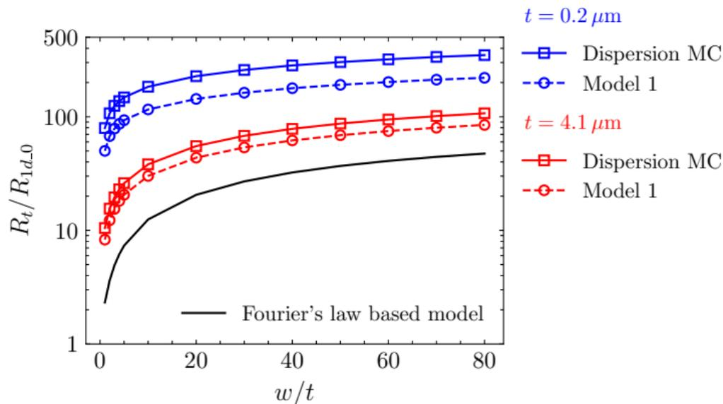
Figure 5: Dimensionless total thermal resistance of GaN as a function of  $w/t$  with  $w_g/w = 0.01$  under different thickness.
