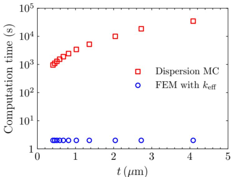
Figure 13: Computation time of Dispersion MC with  $2 \times 10^7$  phonons and FEM with  $k_{\text{eff}}$  as a function of channel thickness using single core.
