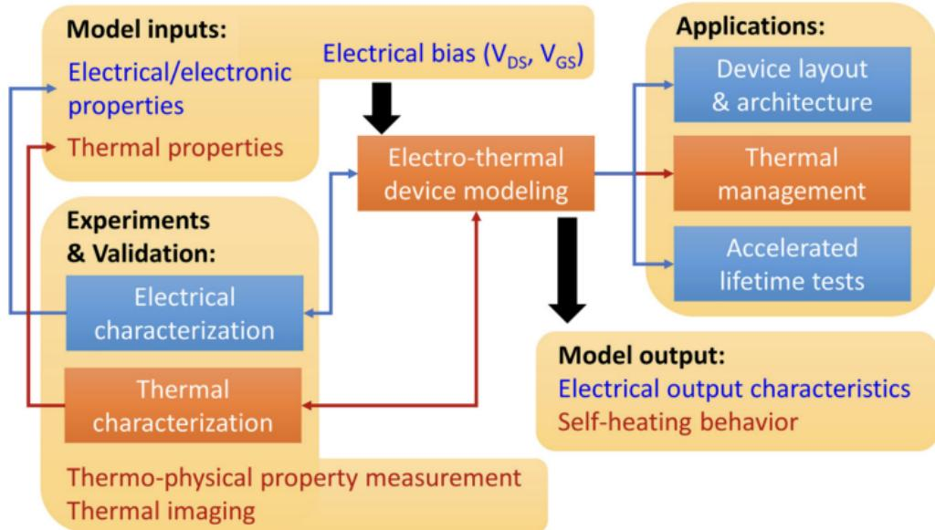
Figure 7: Flow diagram of the device-level electro-thermal co-design process<sup>6</sup>.
