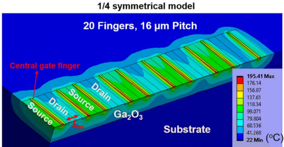
Figure 20: A 3D finite element model for multi-finger transistors<sup>13</sup>.
