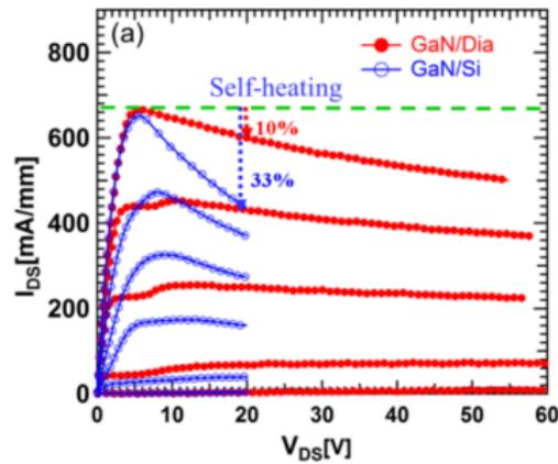
Figure 4:  $I_{DS}$  –  $V_{DS}$  of GaN/Dia and GaN/Si HEMTs<sup>3</sup>.
