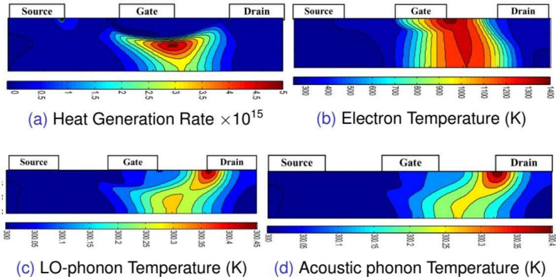
Figure 12: Calculated thermal characteristics in GaN device<sup>9</sup>.
