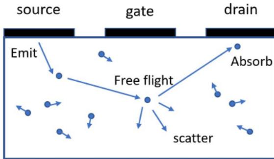
Figure 13: Schematic of electron monte carlo simulation.
