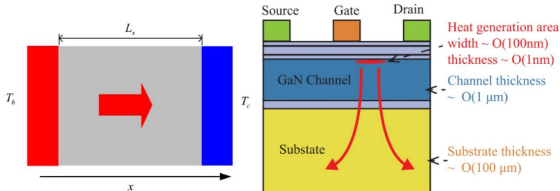
(a) Schematic of measurement of (b) Schematic of heat transport in GaN thermal conductivity of thin films. HEMTs.
