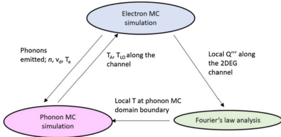
Figure 17: The feedbacks between electron MC simulations, phonon MC simulations, and Fourier's law analysis. The electron and phonon MC simulations are for the transistor region only, whereas the Fourier's law analysis is for the whole sub-mm chip<sup>12</sup>.
