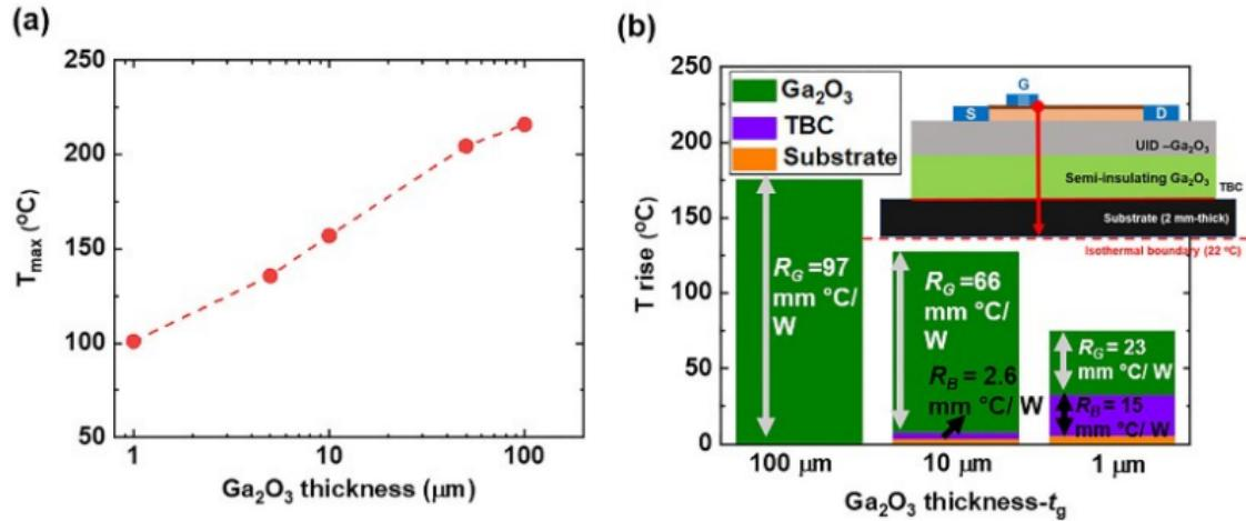
Figure 10: (a) The dependence of channel maximum temperature on  $\text{Ga}_2\text{O}_3$  thickness (b) Modeled temperature rise for the  $\text{Ga}_2\text{O}_3$ -TBC-substrate structure.
