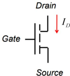
Figure 1: MOSFET circuit symbol.
