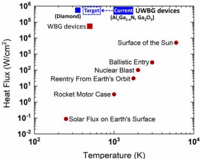
Figure 3: The heat flux challenge of WBG and UWBG power electronic devices (presuming operation at  $\sim 10 \text{ W/mm}$ ).<sup>2</sup>
