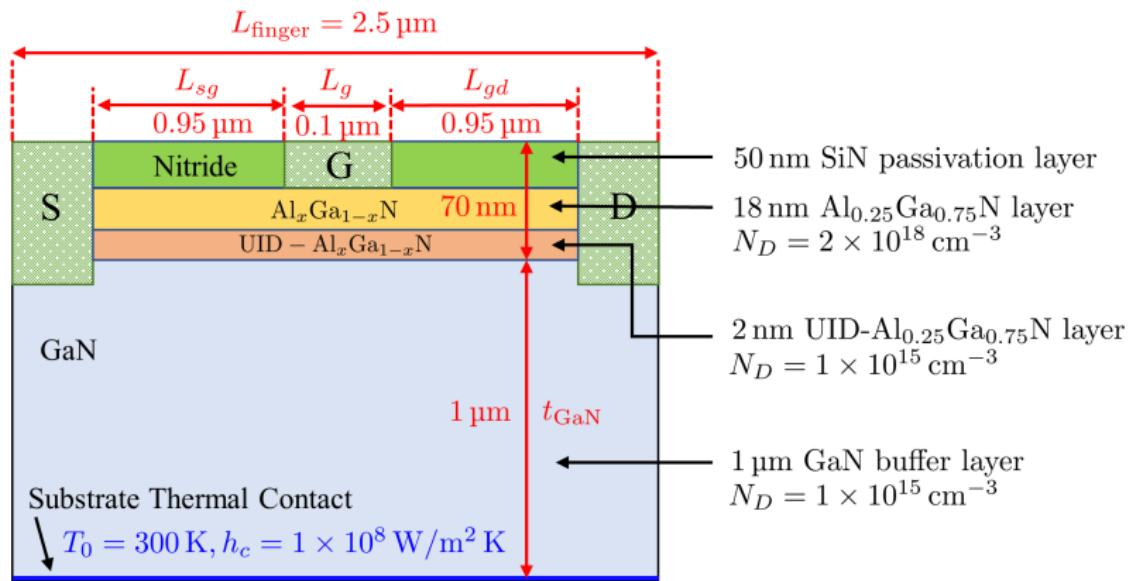
Figure 21: Schematic of GaN HEMT. The geometries are not drawn to scale.
