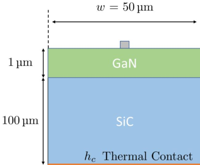
Figure 24: Expected simulated GaN on SiC HEMT.
