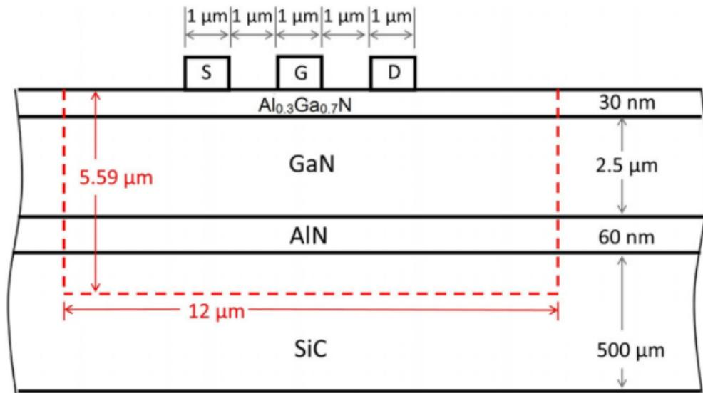
Figure 18: Schematic diagram of the cross section of the simulated GaN HEMT. The region enclosed by the dashed line is the domain for phonon MC simulations.
