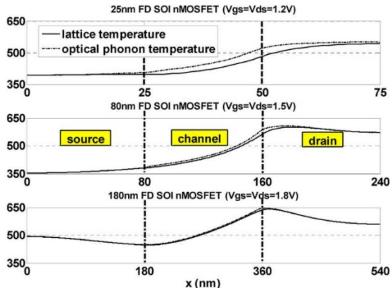
**Figure 15:** Averaged lattice and optical phonon temperature profiles in the channel direction.
