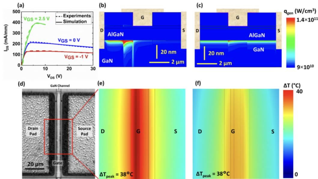
Figure 6: Bias dependent results for channel conditions with  $V_{GS} = -1$  V and  $V_{GS} = 2.5$  V, respectively<sup>5</sup>,  $P_{diss} = 250$  mW.
