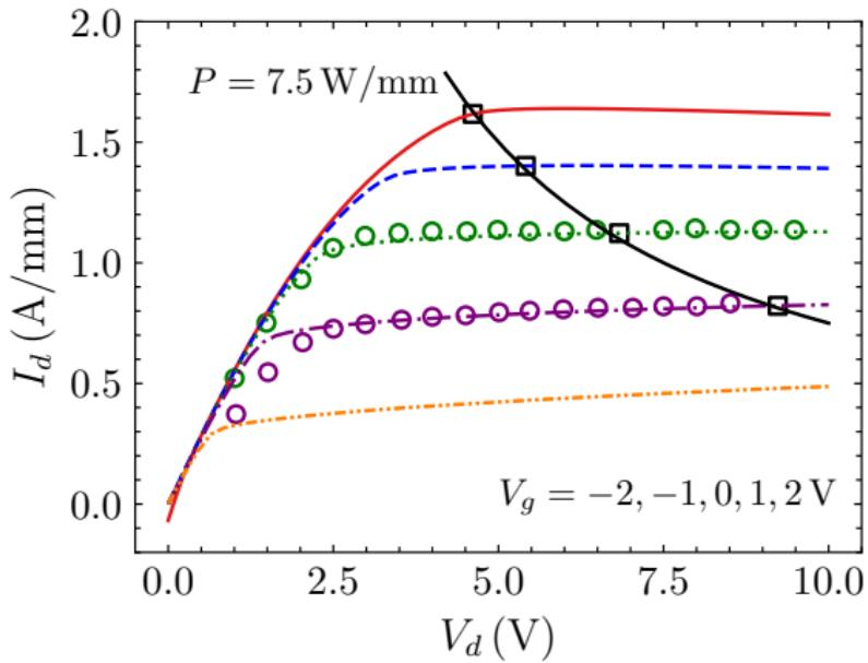
Figure 22: Output characteristics of the HEMT under  $V_g$  from  $-2$  V to  $2$  V with an interval of  $1$  V.
