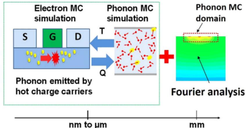
Figure 16: Scheme of multi-length scale electrothermal simulations of a GaN HEMT.
