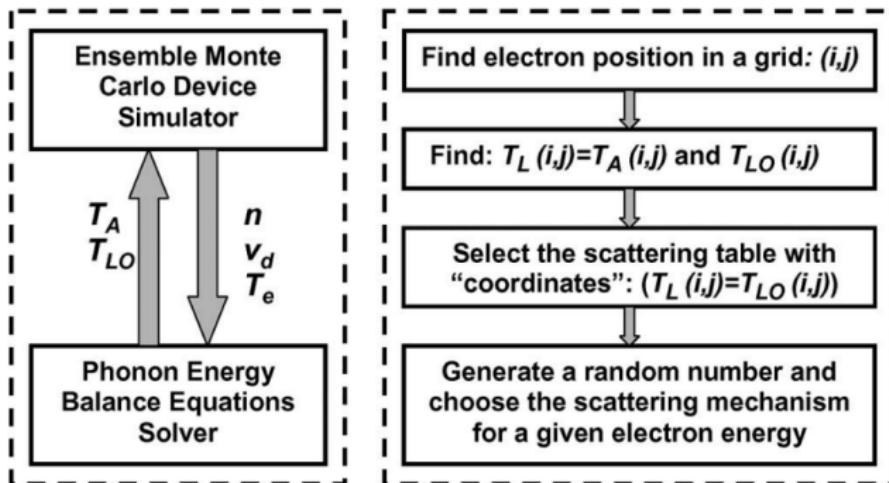
Figure 14: Exchange of variables between the electron system and phonon system.
