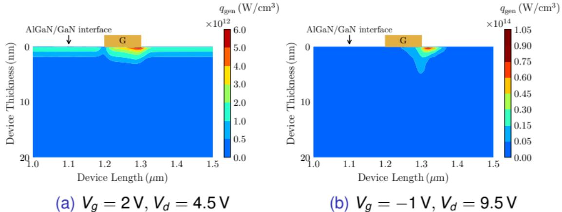
**Figure 23:** The total power dissipation level for the two bias conditions,  $P = 7.5 \text{ W/mm}$ .
