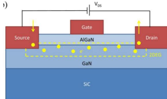
Figure 2: cross-section schematic of HEMT structure <sup>1</sup>.
