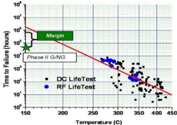
Figure 5: Mean time to failure (MTTF) for TriQuint GaN PAs<sup>4</sup>.
